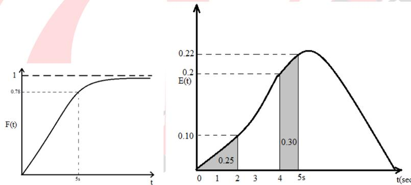
For the same non-ideal reactor, the following E-curve is plotted. The shaded area is given in the shaded region. What is the fraction of tracer that has spent time between 2 sec to 4 sec in the reactor?
