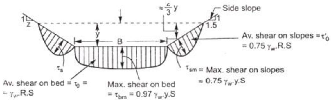
Typical shear stress distribution along the boundary of a trapezoidal channel.
